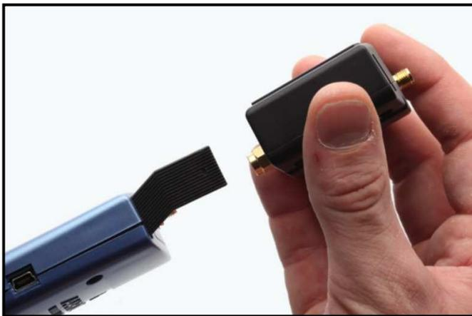
Screw then with enclosed SMA tool the SMA plug of the preamplifier with the SMA jack of the SPECTRAN. Avoid tilting the UBBV-preamplifier in order to avoid damaging the sensitive SMA jacks. Screwing should be carried out very smooth. **Refrain from using force!** As soon as you feel any resistance, please retighten the screw connection. Do this also in a non-violent way! The SMA tool offers a over-tightening protection and starts to slip down if too strong forces are affecting.
