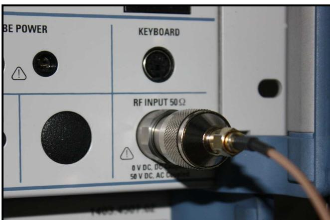
If your measurement unit or antenna is equipped with a N-input, you will need our optional SMA to N adapter as well.
