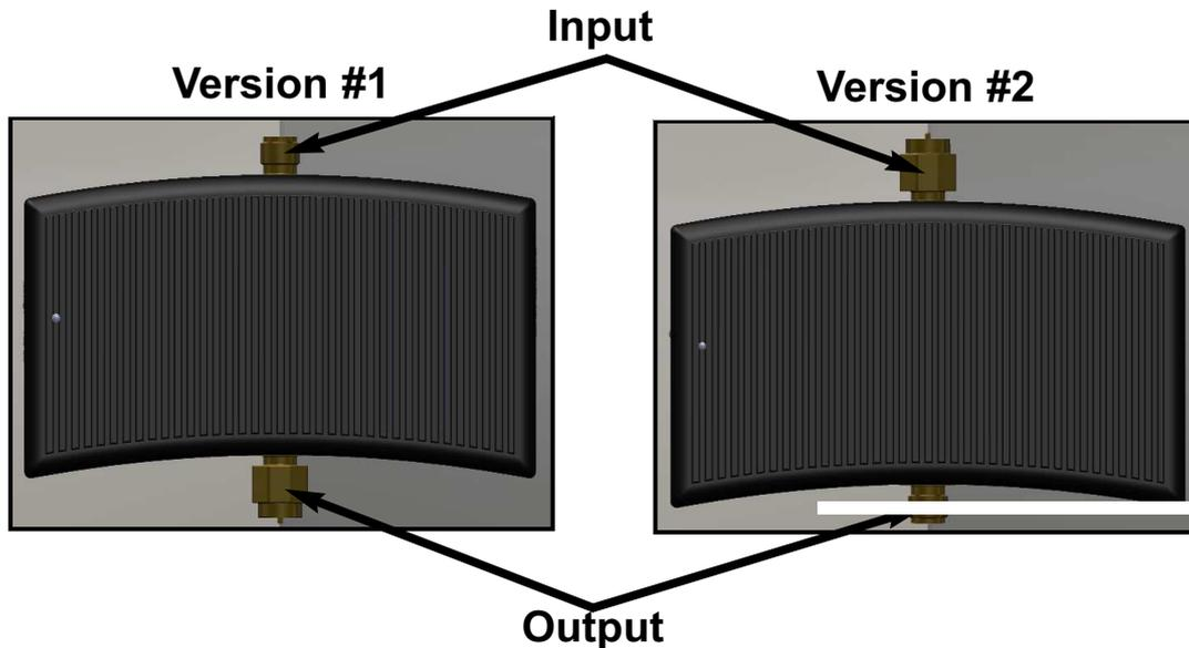
The **output** of the UBBV-preamplifier is always located at the site which is bent inwards.
