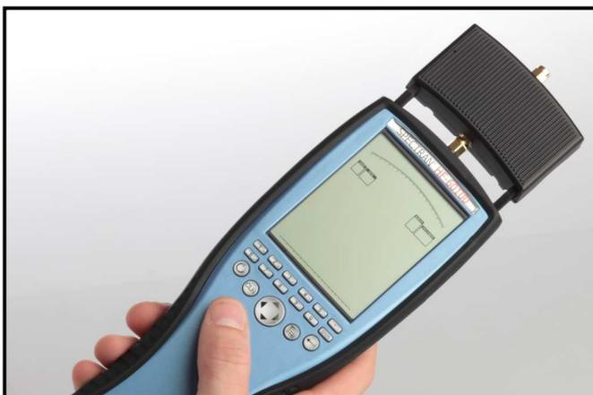
**ATTENTION:** If you don't use the SPECTRAN together with our LCS or MCS software, you have to activate the UBBV-preamplifier in the menu "RefOff" (by choosing the headword "UBBV12") in order that the SPECTRAN is calibrated correctly!
