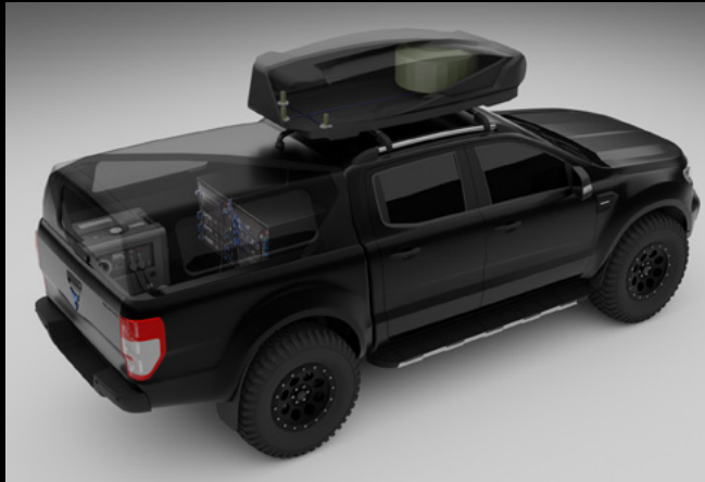
> High-end operator compartment with high resolution displays and server hardware
