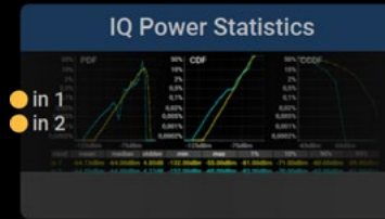
#122/049 Measurement View The IQ Power Statistics block offers a real-time PDF, CDF, CCDF & Relative CCDF statistical RF power measurement.
